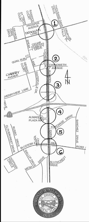
Improvements on this area include construction of sidewalk north of Prosper Avenue and providing a pedestrian friendly square corner at the southwest corner of the intersection for operational benefits. A fourth southbound thru-lane approaching Branham was dropped from the project because right-of-way could not be obtained.
